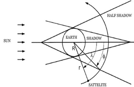
$$\Psi = \begin{cases} 0, & -\phi < \lambda < \Phi \\ 1, & -\pi < \lambda < -\Phi, \Phi < \lambda < \pi \end{cases} \quad (3) \quad \text{Figure 1: Geometry of shadow function.}$$
